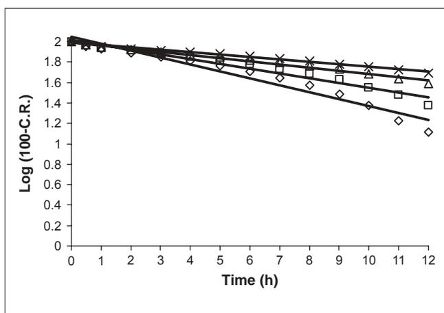
**Figure 5:** First order release profiles of replaglinide from poly( $\epsilon$ -caprolactone) microspheres formulations  $F_1$ ( $\diamond$ ),  $F_2$ ( $\circ$ ),  $F_3$ ( $\Delta$ ) and  $F_4$ ( $\times$ )
